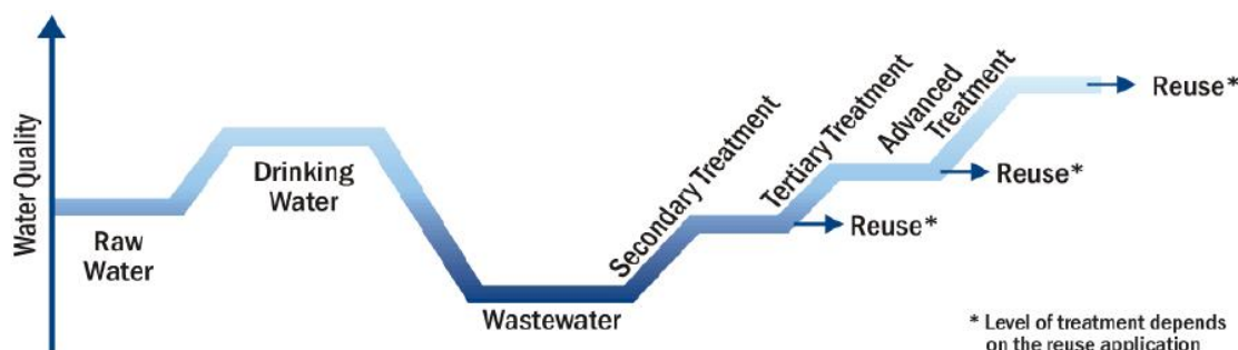
Figure 10.6: Level of wastewater quality
