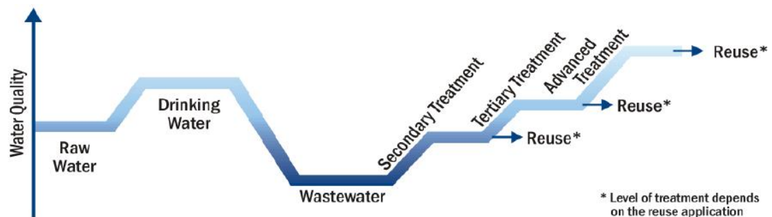
Figure 10.7: Level of wastewater quality
