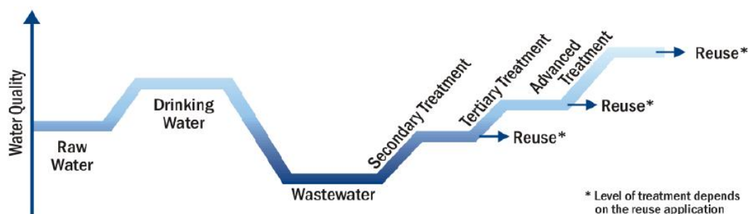
Figure 10.7: Level of wastewater quality
