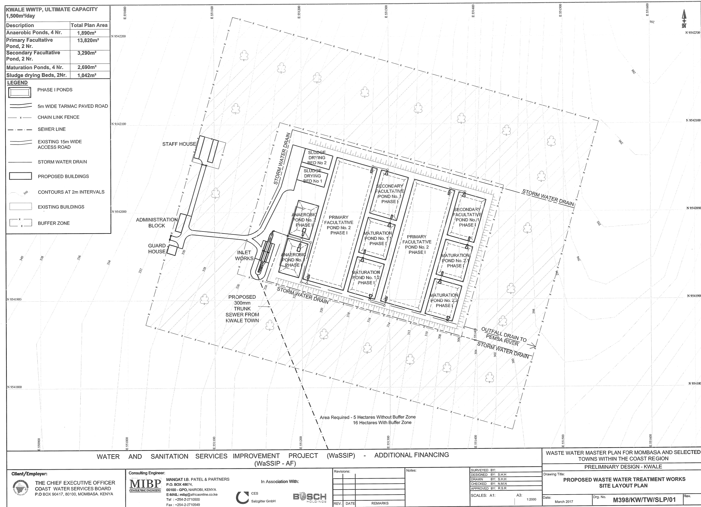
Figure 10.4: Site Layout Plan of the Proposed Waste Water Treatment Plant
